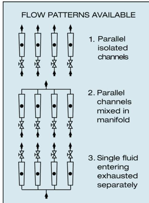
**The built-in-valves are always installed in the end block opposite to the manifolded one.**
